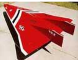
This photo shows the eight-foot-long prototype LoFLYTE, a test vehicle for the Waverider concept. LoFLYTE, which first flew in 1997, has a wing designed to ride on top of its own shockwave. (photo courtesy of ASTRA , which can be reached at info@astra.org.uk )
