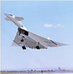
One of the two XB-70 bomber prototypes. The dark lines under the wings, near the wingtips, indicate the places where the wingtips fold down so the aircraft assumes an efficient shape for riding its shock wave. (image courtesy of NASA )
