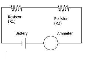
3. Measure and record the voltage across the battery here.
