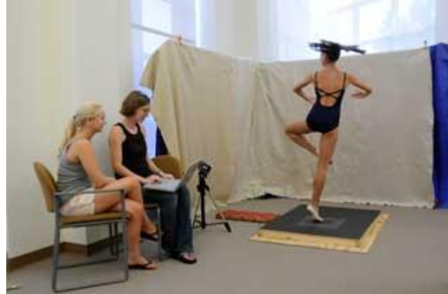
A dancer performing a pirouette on the force platform, while Melanie watches the data on her laptop. Photo credit: Pierce Bounds, Dickinson College
