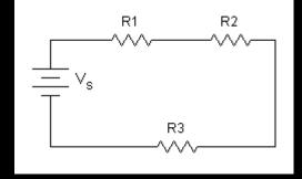
EXAMPLE: If resistors of 2Ω, 3 Ω, and 7 Ω are connected in series in a circuit with a current of 2.5 amps what will be the emf in a source with negligible resistance?
