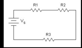
EXAMPLE: If resistors of 2Ω, 3Ω, and 7Ω are connected in series in a circuit with a current of 2.5 amps what will be the emf in a source with negligible resistance?
