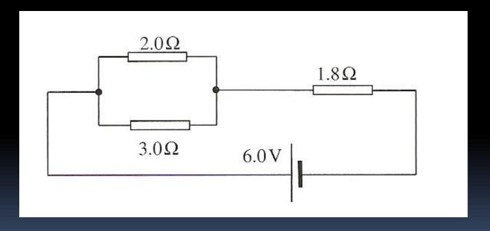
In series resistors, the current through each resistor is the same and the potential difference (drop) is different.
