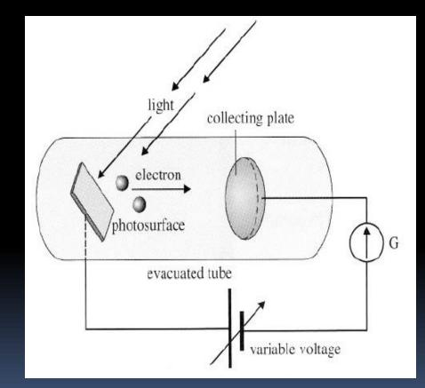
As the intensity of the radiation increases, induced current increases – intensity and current are directly proportional
