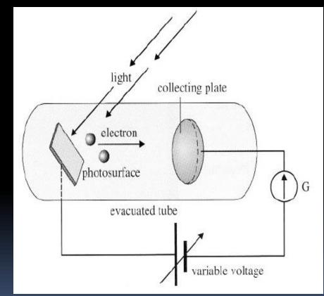
To determine which, you connect up a voltage source to the circuit to make the current drop to zero – a <u>stopping voltage (V<sub>s</sub>)</u>
