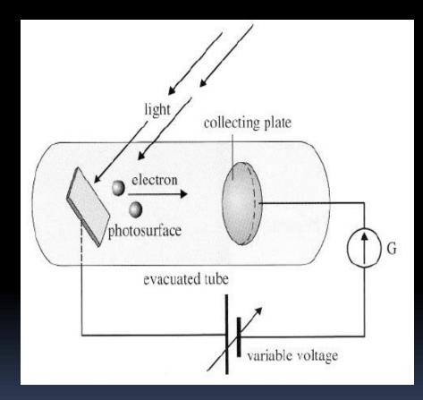
The energy of the stopping voltage, eV<sub>s</sub>, must then be equal to the work done in moving the electrons from the cathode to the collecting plate, which is the same as the maximum kinetic energy of the electrons, Ek
