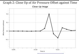
This is a close-up view of the next graph. By clicking on a peak (maximum or minimum intensity offset) the time datum is given. Although there are several data points before the peak (where the ball first hits the table) I used the first maximum or minimum peak (greatest offset intensity) in all the time measurements.
