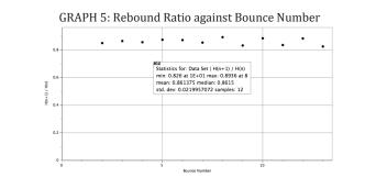
The *LoggerPro* software statistical analysis function tells us the minimum and the maximum values of this rebound ratio. It also tells us the average or mean value, which is 0.861375 or 86.1%.
