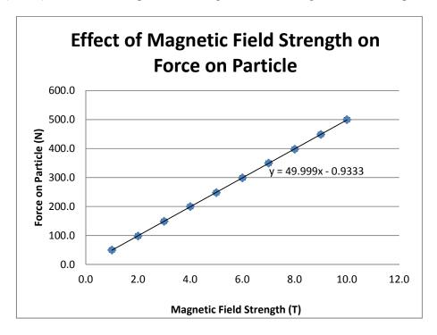
Graph One (data 1): The relationship between magnetic field strength and force on particle.
