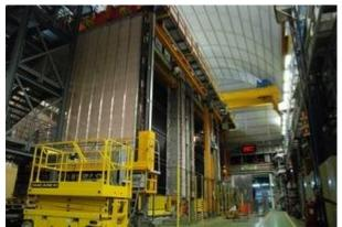
where scientists observe how many of the original muon-neutrinos have transmutated into oscillated tauneutrinos. Shown here is the OPERA detector located in the Gran Sasso underground labs.
