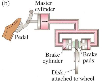
The pressure applied to a confined fluid increases the pressure throughout the fluid by the same amount.
