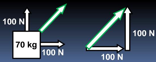
$\Sigma F = \sqrt{100^2 + 100^2}$  $\Sigma F = 141N$  $\Sigma \vec{F} = m\vec{a}$  $\frac{\Sigma \vec{F}}{m} = \vec{a} = \frac{141}{70}$  $|\vec{a}=2m/s^2$  $\theta = 45^{\circ}$
